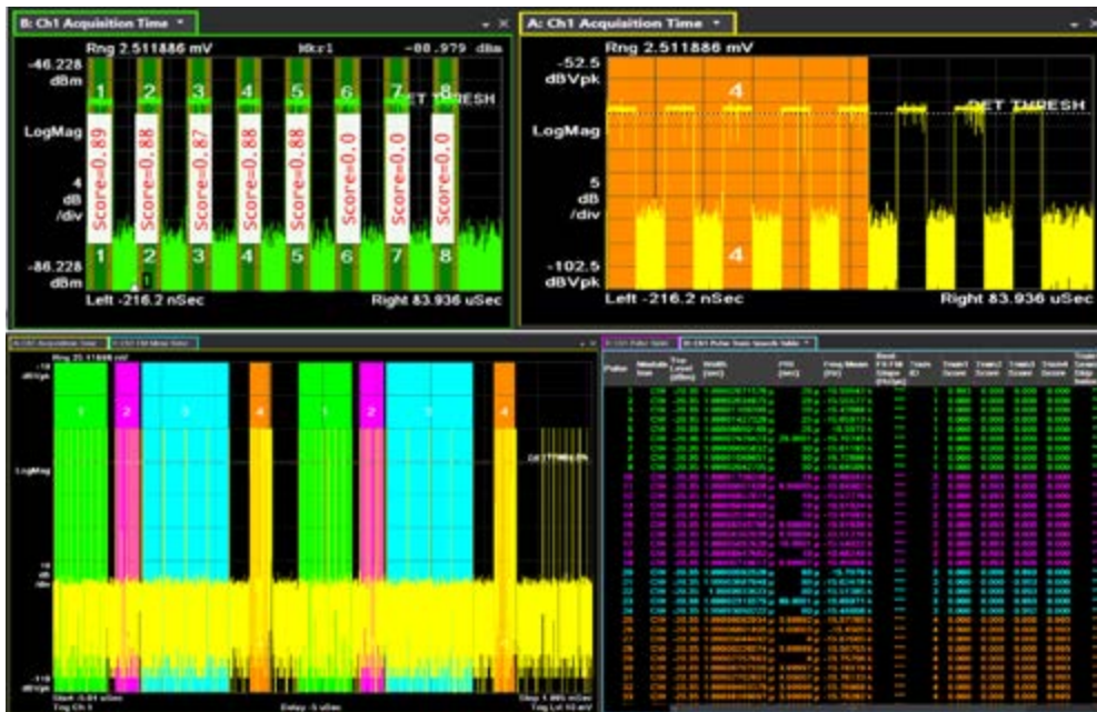
Figure 7. Raster scan shows radar modes and patterns
