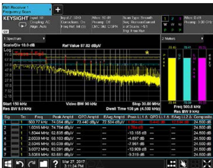
Figure 2.5. When making EMI measurements, you often want to scan and search for signals above the limit.
