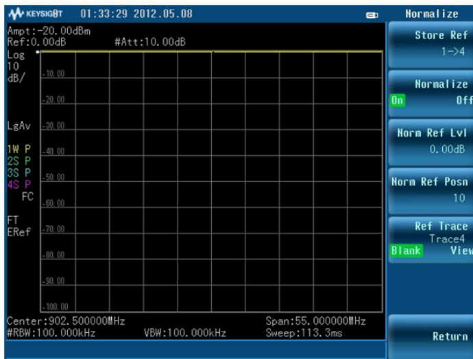
Figure 6. Normalization establishes a 0-dB reference trace
